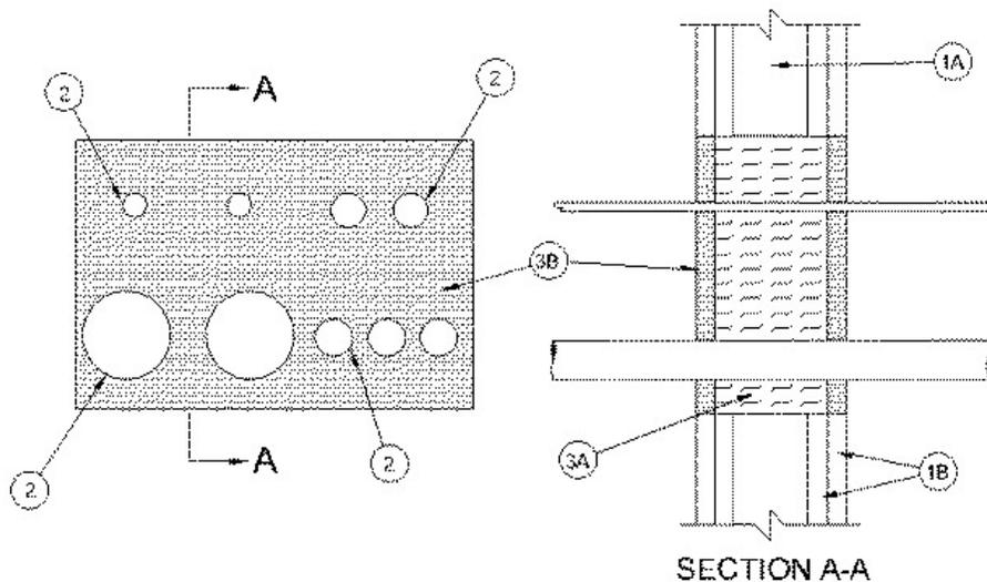
**1. Wall Assembly** — The 1 or 2 hr fire-rated gypsum board/stud wall assembly shall be constructed of the materials and in the manner specified in the individual U300, U400, V400 or W400 Series Wall and Partition Designs in the UL Fire Resistance Directory and shall include the following construction features:
