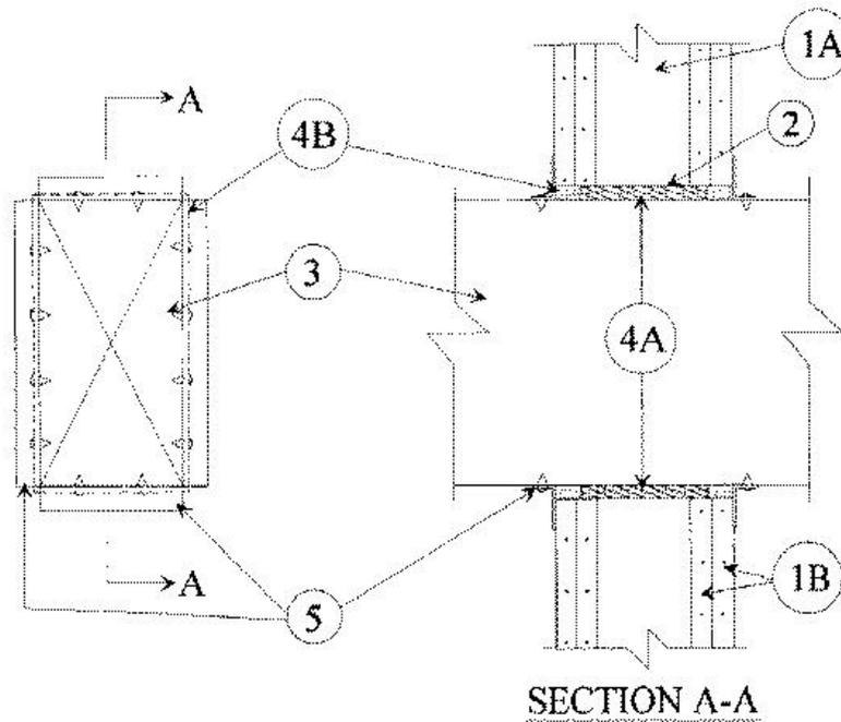
**1. Wall Assembly** — The 1 or 2 h fire-rated gypsum wallboard/stud wall assembly shall be constructed of the materials and in the manner specified in the individual U300 or U400 Series Wall and Partition Designs in the UL Fire Resistance Directory and shall include the following construction features:
