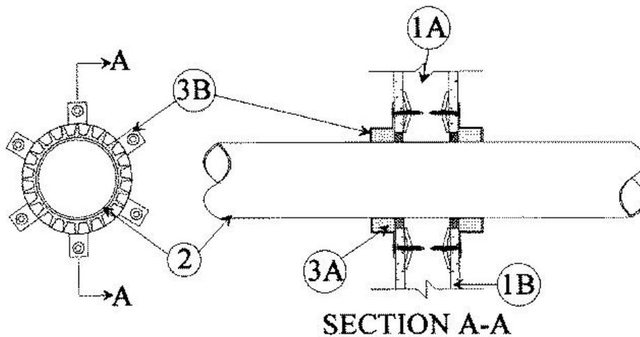
**1. Wall Assembly** — The fire-rated gypsum wallboard/stud wall assembly shall be constructed of the materials and in the manner specified in the individual U300 or U400 Series Wall and Partition Designs in the UL Fire Resistance Directory and shall include the following construction features:
