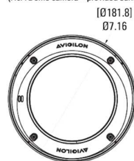
Dome Camera with Surface Mount (H6A Dome camera + provided surface mount)
