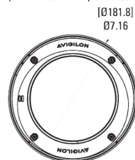
Dome Camera with Surface Mount (H6A Dome camera + provided surface mount)
